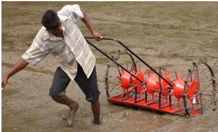
Figure 3. Initial design of conical drum seeder.
