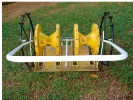
Figure 7. Adjustable conical shape drum seeder.
