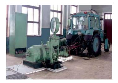
Test engine power up to 400 kW
