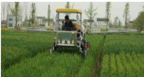
Machine-mounted devices for crop growth monitoring and diagnosis
