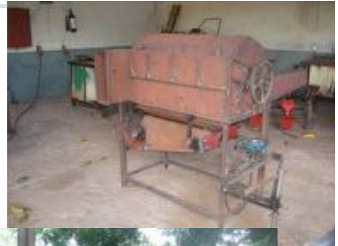
Multi-crop thresher with cleaning device
