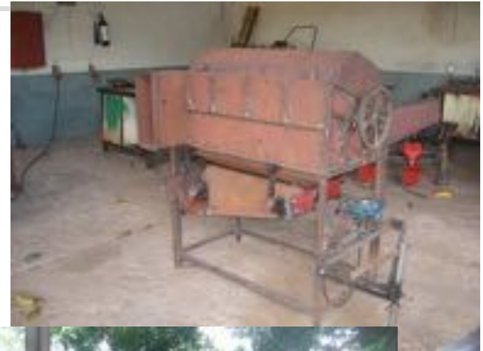
Multi-crop thresher with cleaning device
