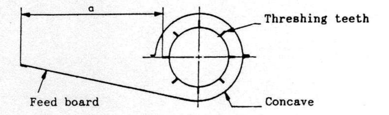
Figure 4 Normal distance from threshing teeth to feed board (clause 4.1.1)
