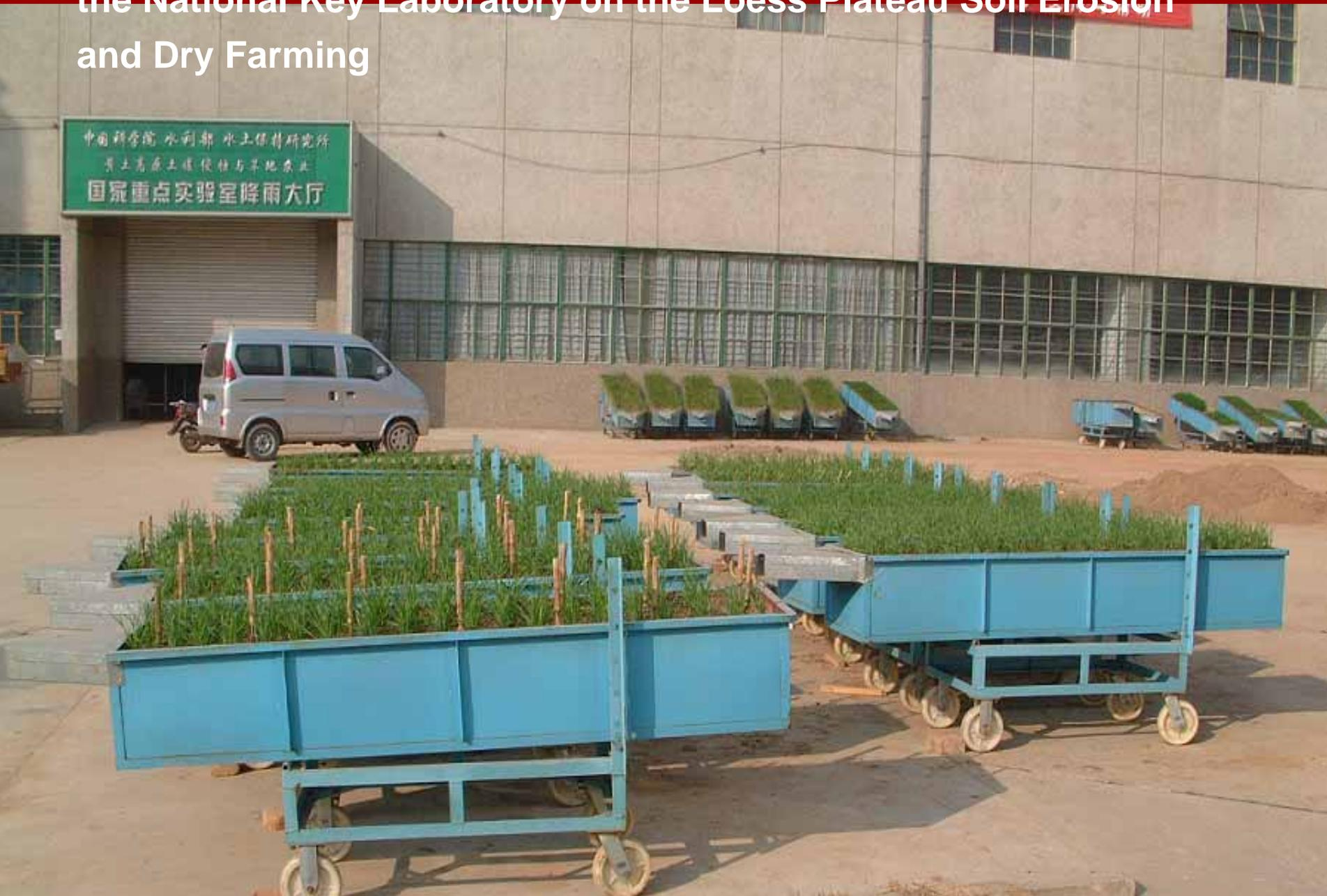
➤ Using side gush automatic simulated rainfall system, the sprinkler is 16 above, its velocity was 98% the amount of that natural raindrop arrived to the land. The rainfall intensity was 120mm/h, and the time was 60 min.
