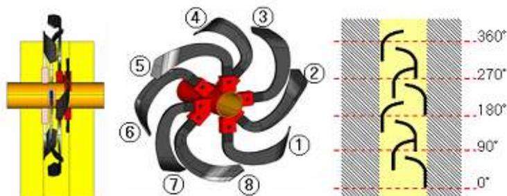
(a) Top view (b) Isometric view (c) Sequence of soil cutting
