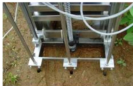
Fig. 1. Digital soil strength measuring device
