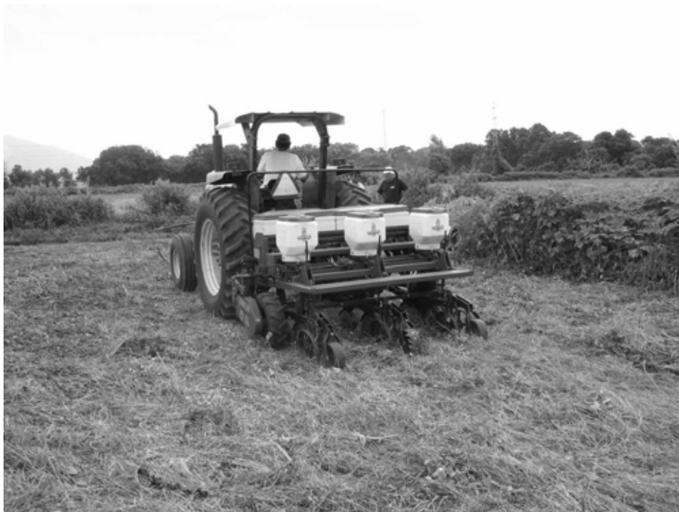
Picture 2: Direct seeding with minimal soil movement into heavy mulch cover (photo Friedrich)
