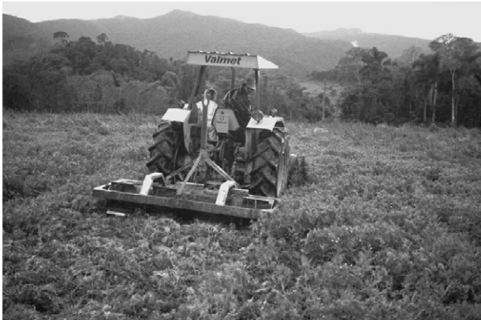
Picture 1: Knife roller used for rolling down a covercrop (photo Friedrich)
