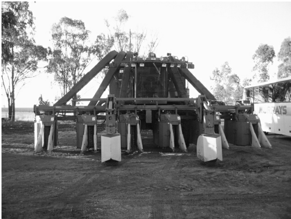
Picture 4: 6-row cotton picker adapted for controlled traffic farming at 3 m track width; additional support wheels in the front have been constructed by the farmer to support the header weight without double tyres (Jamie Grant/Australia) (photo Friedrich)
