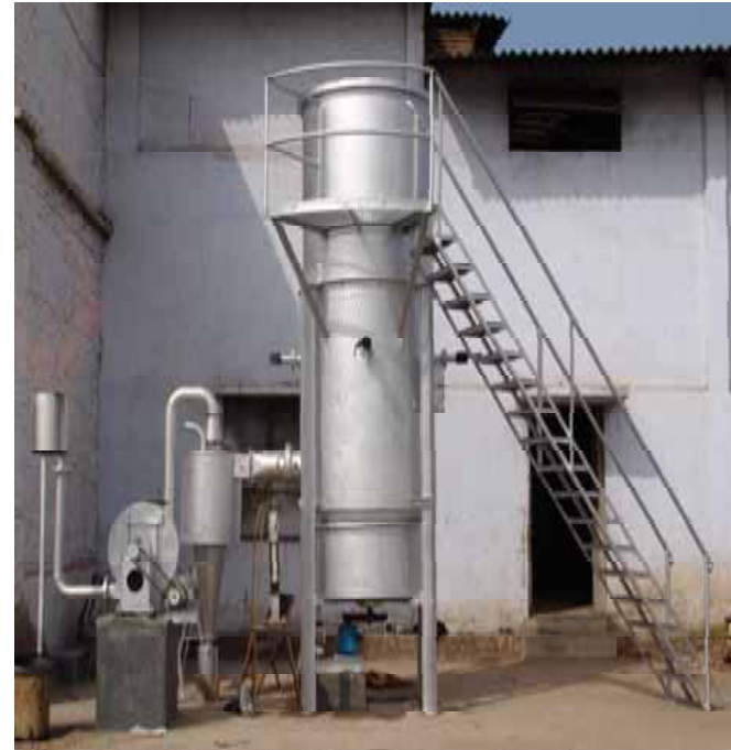
Producer gas system installed in an industry near Anand (Gujarat) for chicory roasting
