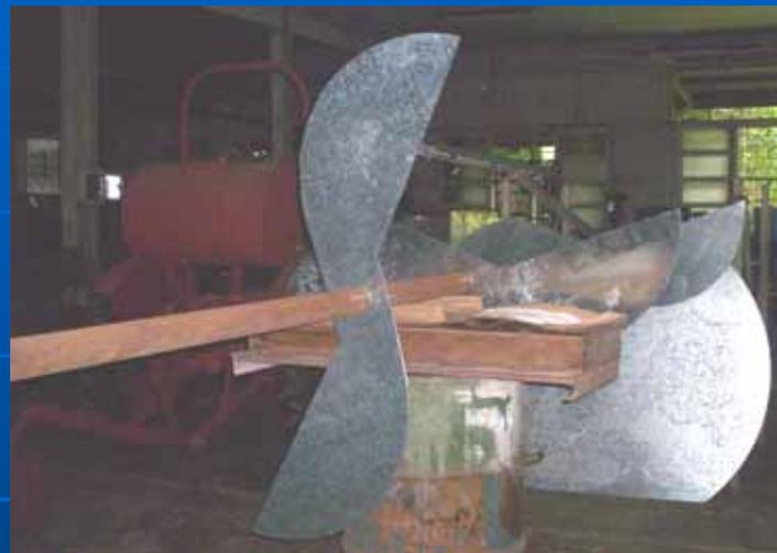
Fabricated parts of the proposed S-rotor Bach-type windmill for pumping purposes.
