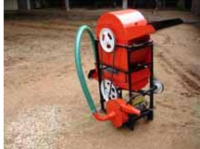
Two type of decorticators can shell the groundnut for consumption and also for seeds. Manual operated machine has the capacity of about 50 kg per hour and the electrical motor driven machine has fairly a large capacity.
