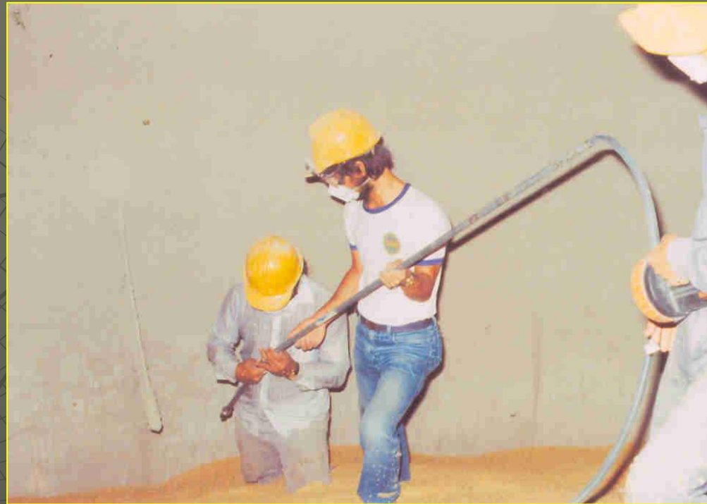
Paddy sampling inside the concrete silo
