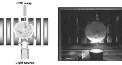
Figure 4.7. Arragement of light and detector for sugar sorting of Satsuma mandarin
