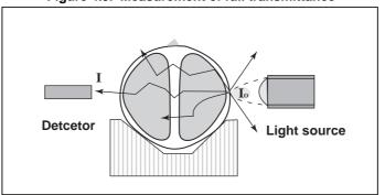
Figure 4.5. Measurement of full transmittance
