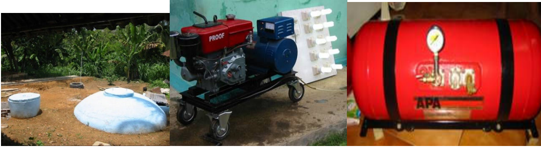
Figure 4. Biogas reactor, dual-fuel engine for electric generator and biogas bottling
