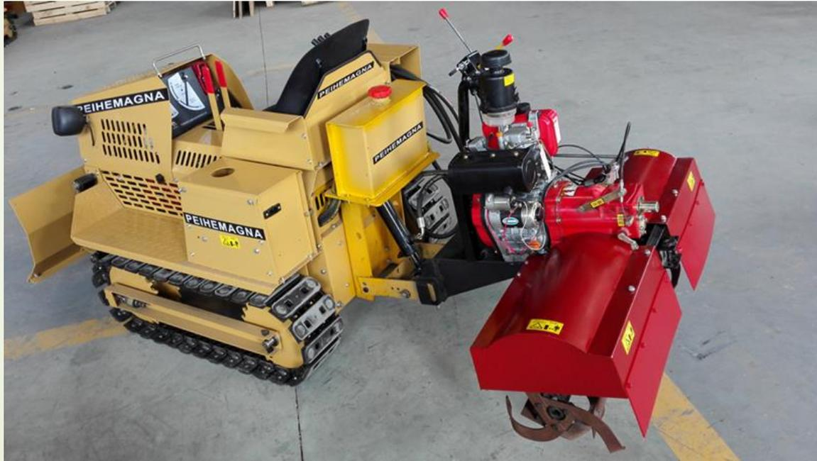
This machine is designed to cope with the complex conditions of farmland in the mountainous area. Use of cartridge design, can be replaced within a few minutes to achieve a multi-purpose machines, reduce cost of purchasing machines for small holder farmers.
