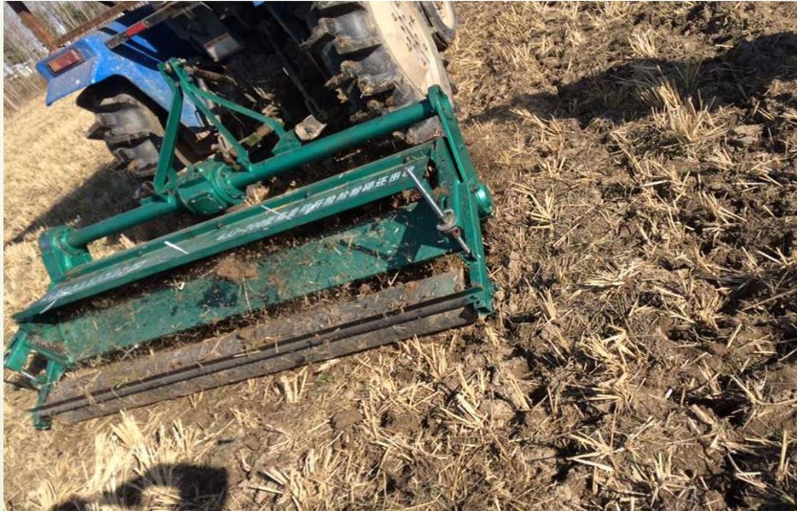
This machine is used to cut up straw and mix straw with soil, it can effectively reduce the burning of straw and increase the organic matter in soil, improve the soil structure, make crop grow more stalmart.
