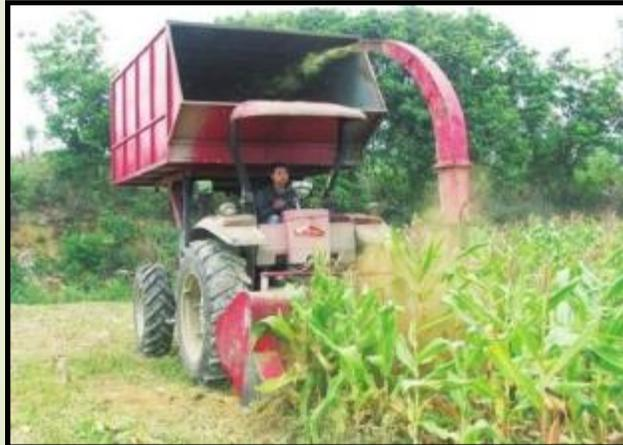
Self-propelled silage harvester
