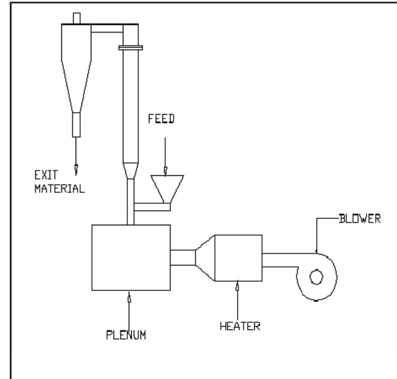
Schematic diagram of the AMDP Pneumatic Dryer
