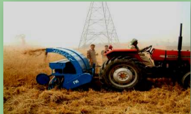
Seeder For Combined Harvested Paddy Fields
