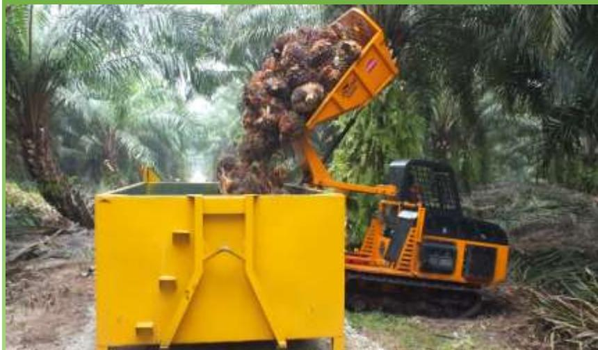
*Jaguar X800, a 37HP multipurpose tractor was designed with a single chassis, compact and robust with the most efficient weight distribution ratio and the least ground pressure.*
