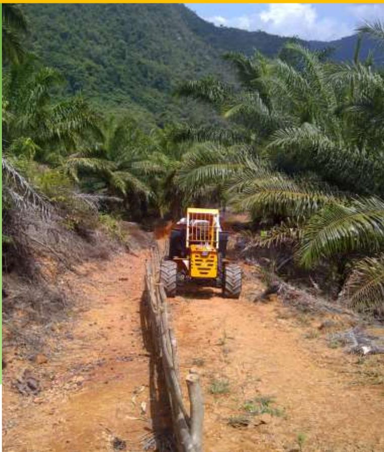
Rhyno is capable of carrying 700 kg of FFB payload, utilizing a minimal diesel fuel consumption of only 6-8 litres a day.
