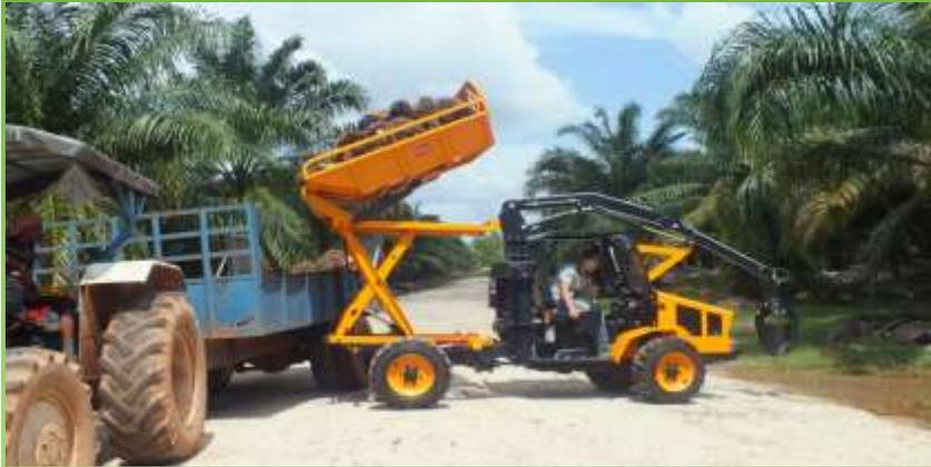
Tiger G1500 is capable of carrying 1500 kg of FFB payload, utilizing a minimal diesel fuel consumption of only 12 litres a day.
