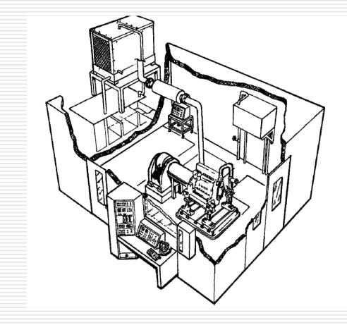
General purpose test cell arranged against an outside wall with control desk 'side on' to engine
