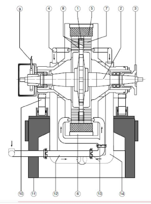
Schenck Dry gap, Disc type Eddy current dynamometer 1. Rotor, 2. Rotor Shaft,3. Coupling flange, 4. water outlet with thermostat,5.Excitation coil,6. Dynamometer housing,7. Cooling chamber,8. Air gap, 9. speed pickup,10,Flexure support, 11. Base,12. water inlet, 13. Joint, 14. water outlet pipe.
