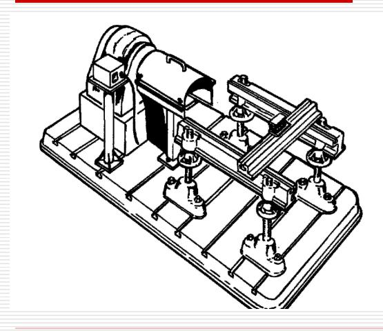
Dynamometer and engine mounting stand on a common tee-slot bedplate. This type of stand, requiring crane loading of the engine.
