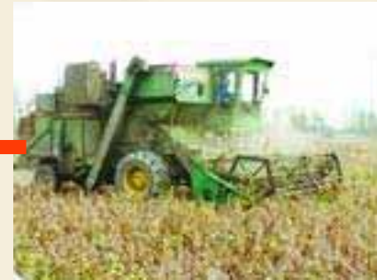
Combine harvest soybean Stalk smashed and covered
