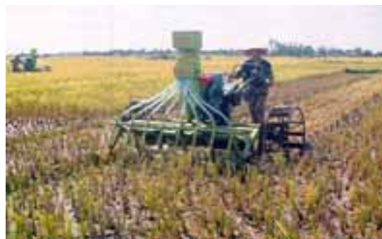
Fig. 1. Sowing soybeans directly to the rice field without tillage, just after rice harvested
