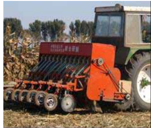
Fig .5 2BMDF-12 No-Till Wheat Seeder.
