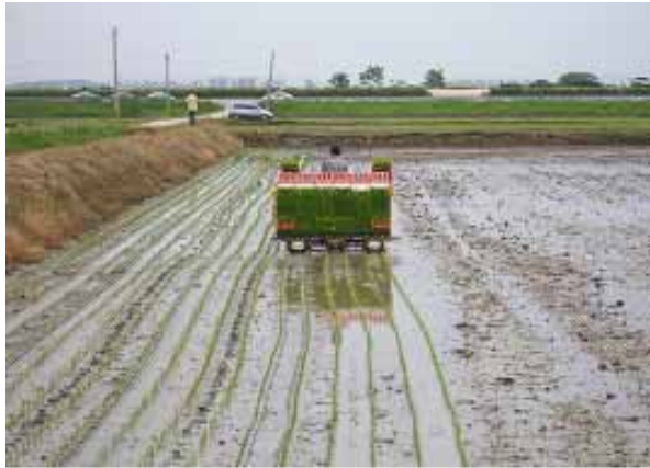
Fig.2 Map-based variable fertilizer applicator attachable to a transplanter
