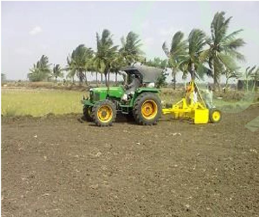
“ If land leveling is done with the use of laser guided land leveler both in lowland and highland about 20% - 30% water can be saved and also crop growing will be in uniform. The laser guider has to be imported and preliminary trials will be conducted.
