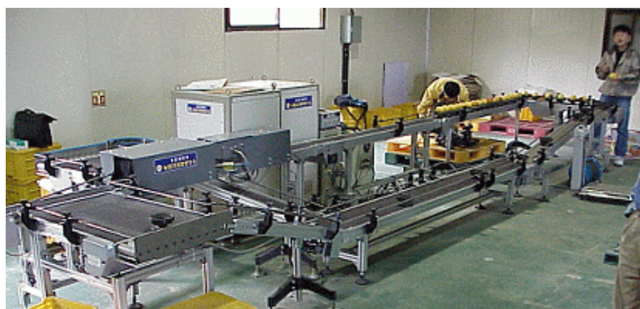
Fig. 7 Peach grading system by sugar content.
