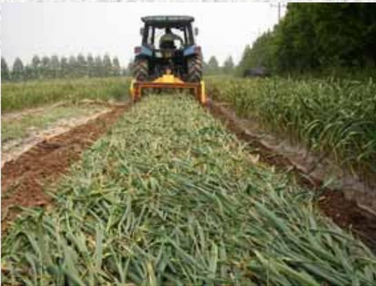
◀ A garlic digger mounted on tractor that can harvest seed garlic produced from bulbils or regular garlic bulb
