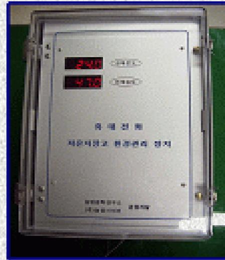
▲ Environmental control device for cold storage house using mobile phone
