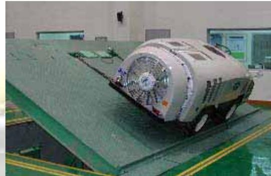
▲ Executing the turn-over test of off-road vehicles. The inspection of turn-over angle is performed by the local test method.
