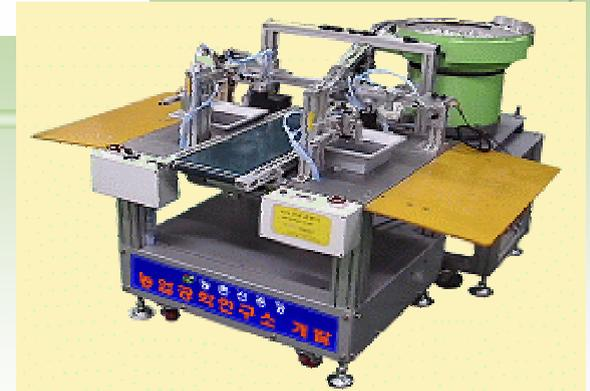
▲ Grafting machine which can automatically carry out the series process such as cutting, joining, clipping, discharging for grafting gourd family vegetables
