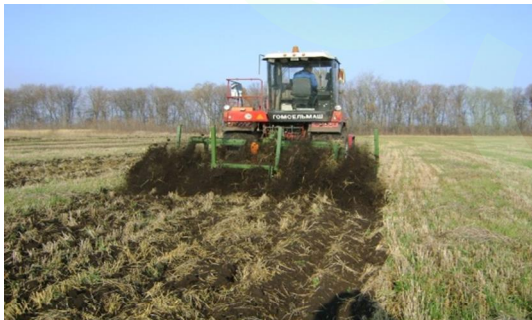
Rotary chisel plow for depth of 45-50 cm
