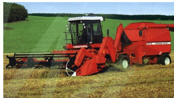
Grain harvester complex KZR-10“Polesje” Rotor” with front mounted header and axial rotary thresh drum-separator also fastened behind to UES by the block of air-cleaning with a grain bunker. - productivity on a grain up to 20 t/hr
