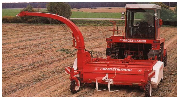
Sugar-beet harvester KSN-6 “Polesje” for one pass cuts tops, digs out, cleans and stacks roots in a row between wheels of power unit. - productivity up to 2 hectare/hr
