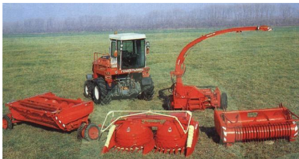
Forage harvester complex K-G-6 “Polesje” with chopper and adapters for cutting green grasses, haylage and silage from grasses and corn. -productivity up to 90 t/hr
