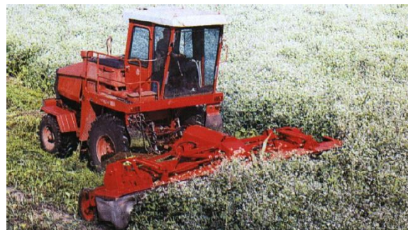
Rotary mower-crusher KPR-6 “Polesje” with demountable conditioners for crushing of grasses and stacking two swaths. - productivity up to 6 hectare/hr
