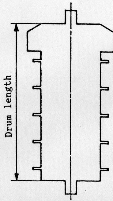
Figure.1 Length of threshing drum
