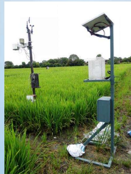
Figure 3: EWS system for pest outbreak monitoring
