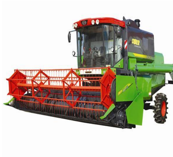
Whole-feed combine harvester, wheeled Rating throughput: 10kg/s
