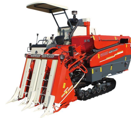
head-feed combine harvester, Tracked working rows: 2 rows
