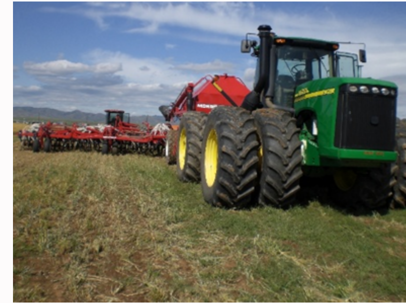
JD 9430 tractor (engine power 439 HP) and Air seeder MAXIM II
