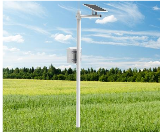
土壤环境监测设备 Soil environment monitoring equipment
