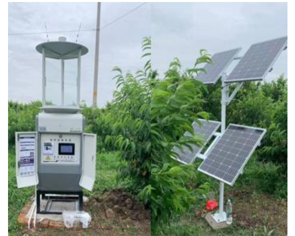
物联网虫情测报灯 Internet of Things (IoT) Insect Detection Lights
