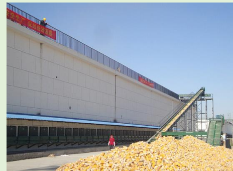
Stacked corn ear drying chamber with slopping bed
