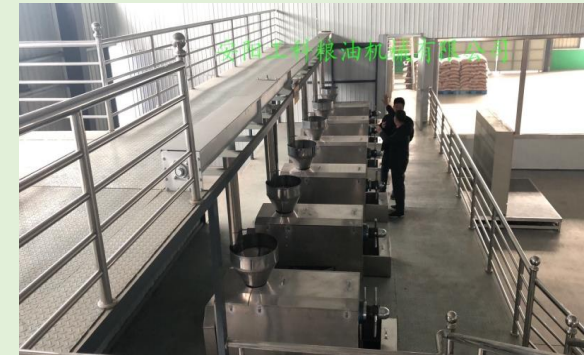
100T/D soybean Oil pressing equipment
