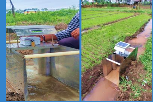
IoT-enabled flume in open channel flow measurement
