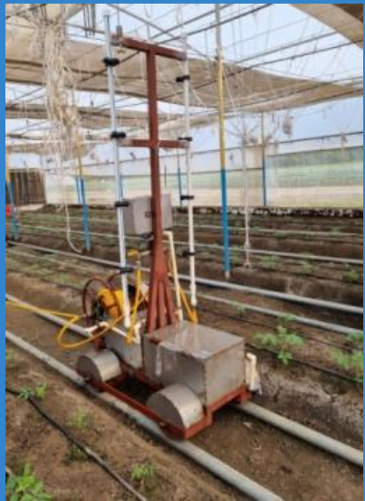
Automatic spraying system for polyhouse
