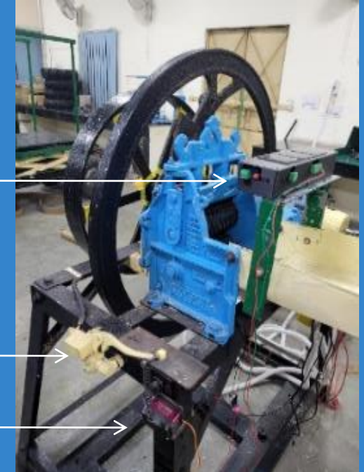
Sensor-based braking system for powered chaff cutter using PIR sensor
