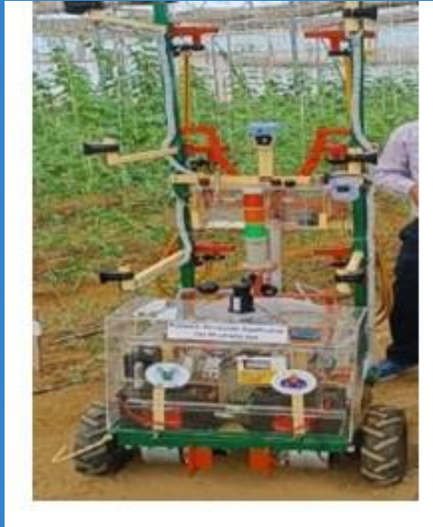
Robot for pollinator and spraying operation in greenhouse
